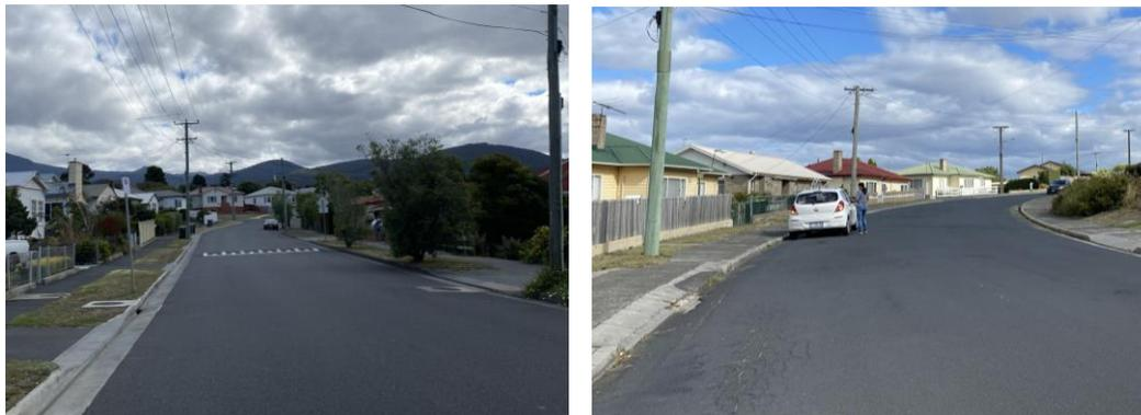
Figure 11: Traffic calming measures in residential areas (left), and large stretches of unrestricted kerbside parking (right)
