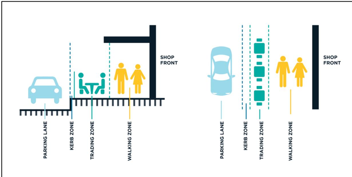
The **kerb zone** is a minimum of 0.6m from the vertical face of the kerb to allow for access to and from parked vehicles and to provide separation between the trading zone and traffic. At an accessible parking space this shall be increased to 1.5m and at a loading zone to 1m.
