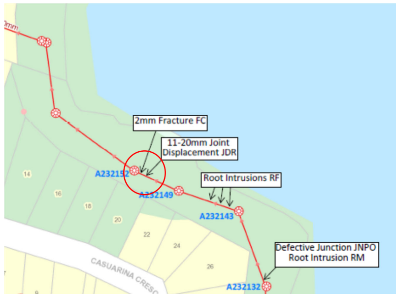
Figure 6 – location of Point 2 close to cracked mains sewer, circled in red
