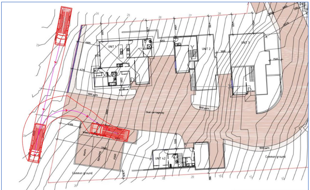
Diagram 8.7 – Swept path of a reversing SRV into a designated waste collection space
