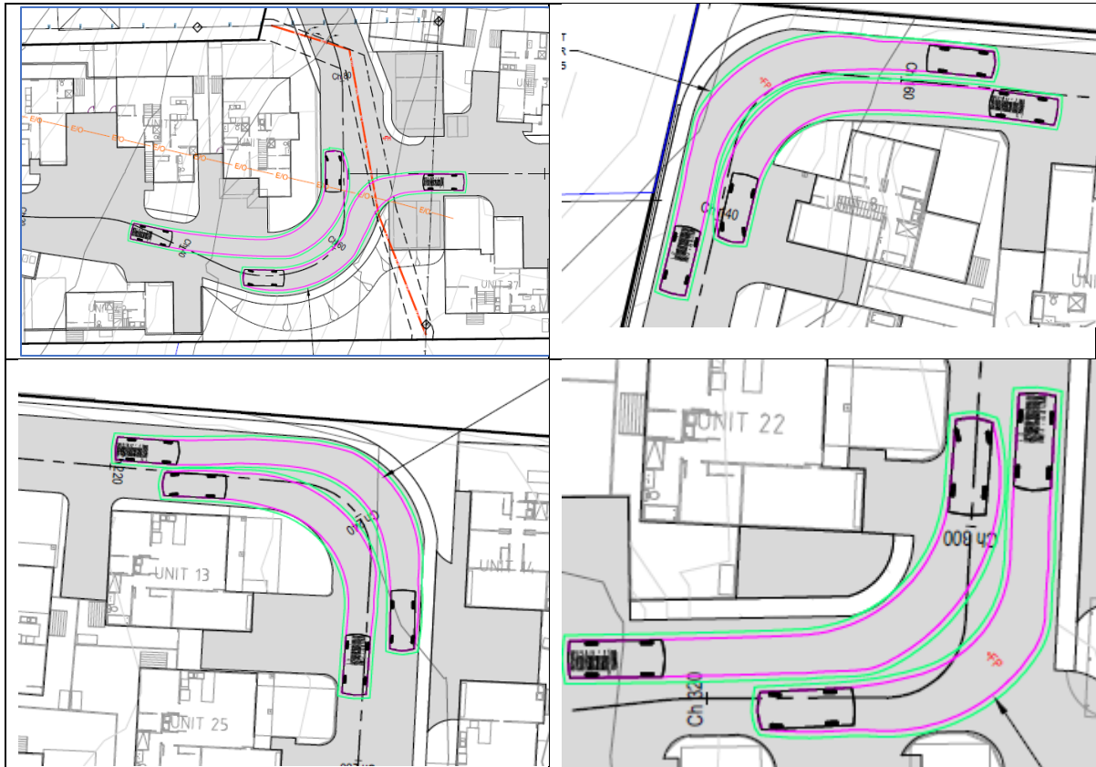
Diagram 8.11 – Curve widening to facilitate two-way vehicle movements
