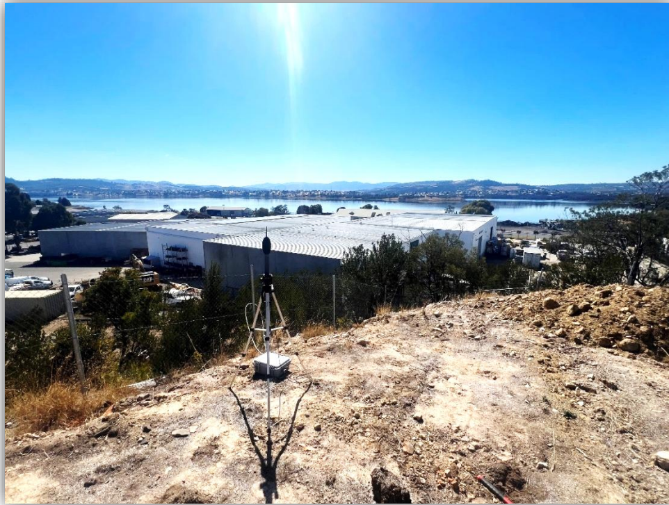
Figure 3-2: Photograph of the SLM at the measurement location, view to the north (by Tarkarri Engineering).
