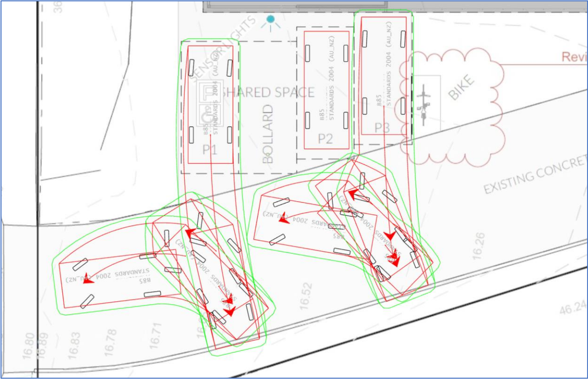
Swept path of a B85 vehicle leaving the 90 degree spaces – third parking module
