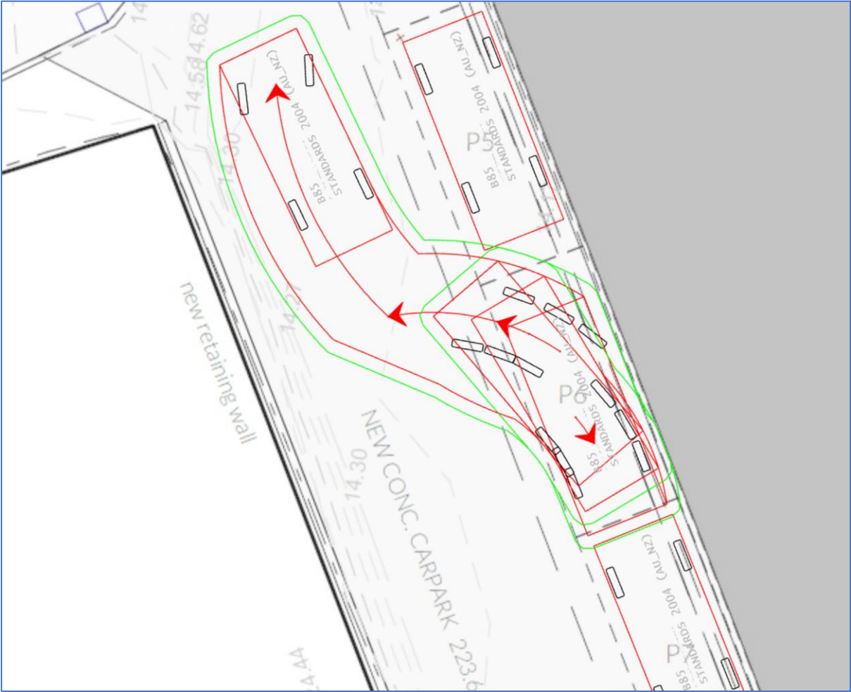
Swept path of B85 vehicle leaving the parallel spaces – second parking module
