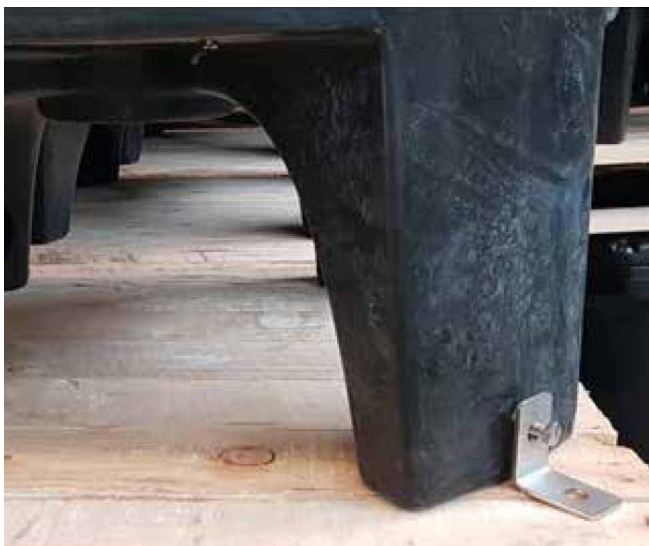
Figure 4 - Bolting the feet.
